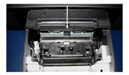
Pay attention not to damage the paper end sensor when cleaning the print head.
