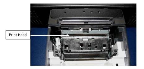
Clean print head and rubber roller with a soft lint-free cloth moistened with pure Isopropyl alcohol (e.g. ISOPADS which can be ordered from Wincor Nixdorf).
