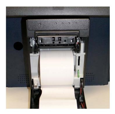
Lay the unwinded paper over the front edge of the printer and close the printer cover. Press on the middle of the cover until it audibly and distinctly locks into place.
